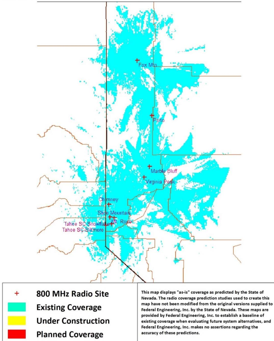
**Figure 4 – Existing 800 MHz NSRS Mobile Radio Talk-out Coverage from Washoe County sites**
