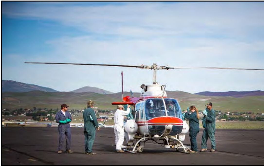
Figure 4. Vector-Borne Disease Program staff load granular mosquito larvicides into helicopter. The typical load amount is five 40-pound bags per side. The helicopter can treat approximately 160 acres per hour depending on climate variability and product treatment rates.
