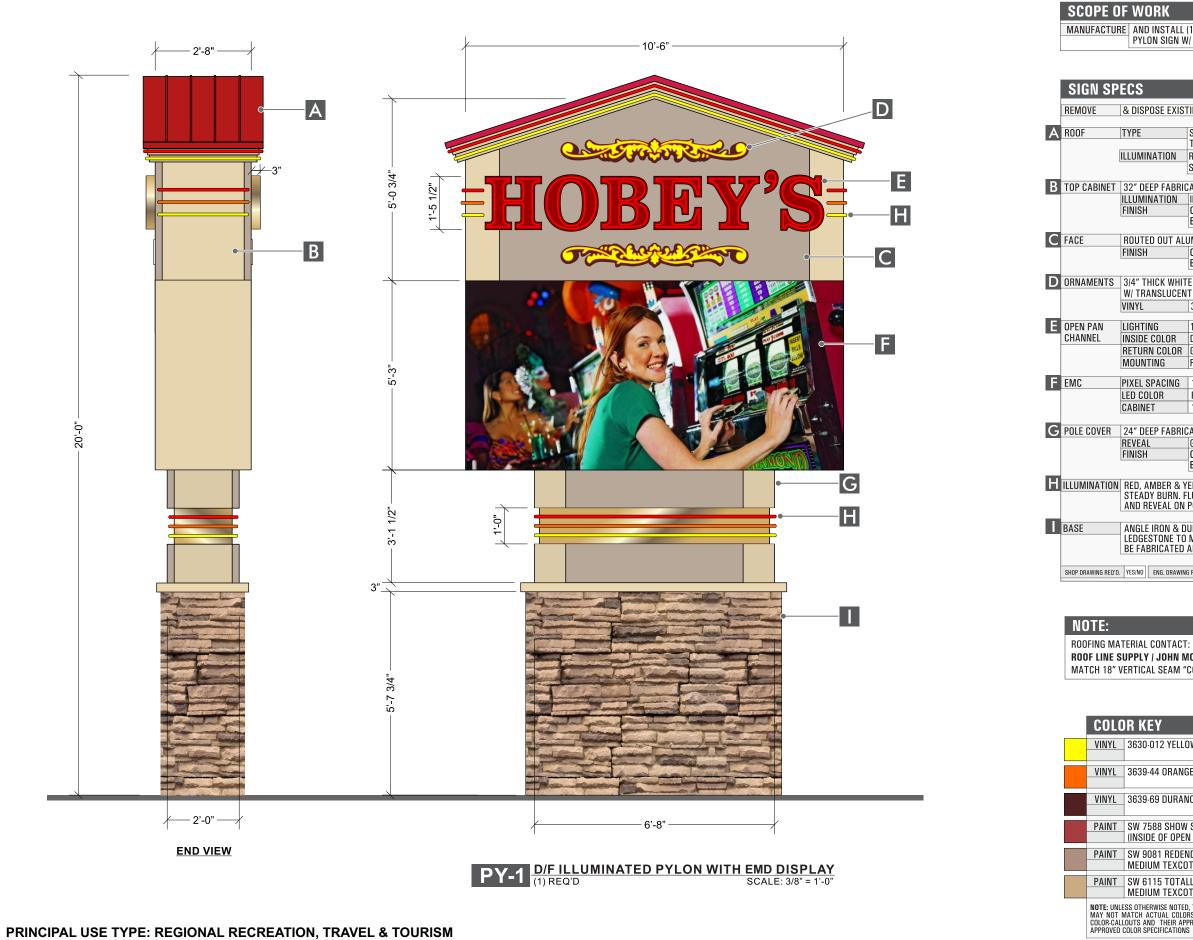
MANUFACTURE AND INSTALL (1) ONE D/F ILLUMINATED PYLON SIGN W/ LED DISPLAY.
