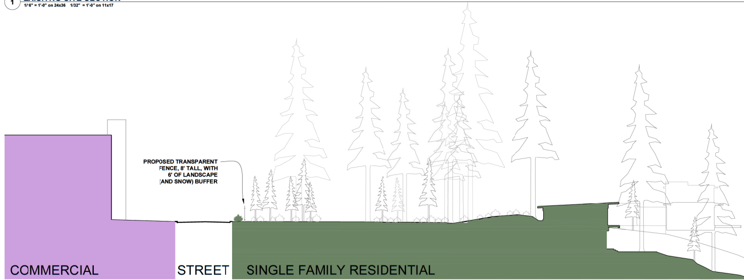
2 SITE SECTION SHOWING PROPOSED FENCE & LANDSCAPE BUFFER 1/8" = 1'-0" on 24x36 1/32" = 1'-0" on 11x17
