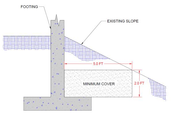
Figure 3: Typical Footing Embedment Diagram Adjacent to Slopes
