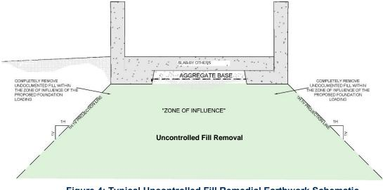
Figure 4: Typical Uncontrolled Fill Remedial Earthwork Schematic
