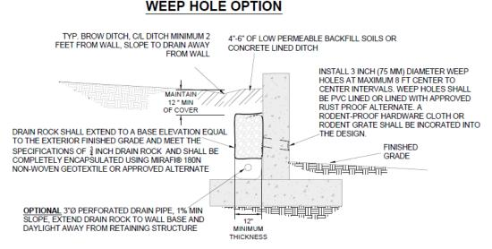
Figure 7: Option 2 Typical Non-Basement Retaining Wall Back-of-Wall Drainage Schematic
