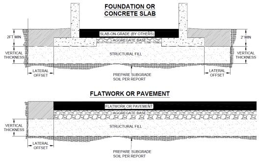
Figure 5: Vertical and Lateral Offset from Potentially Expansive Soil Schematic
