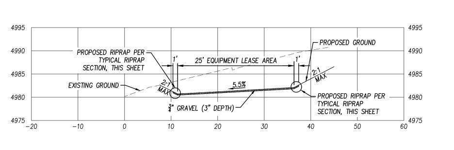
SECTION B-B HORIZONTAL SCALE: 1"=10' VERTICAL SCALE: 1"=10'
