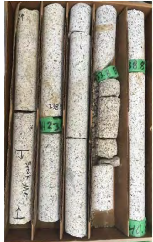
Granitic Bedrock Cores Boring B-09, 20.5 to 40.8 Feet
