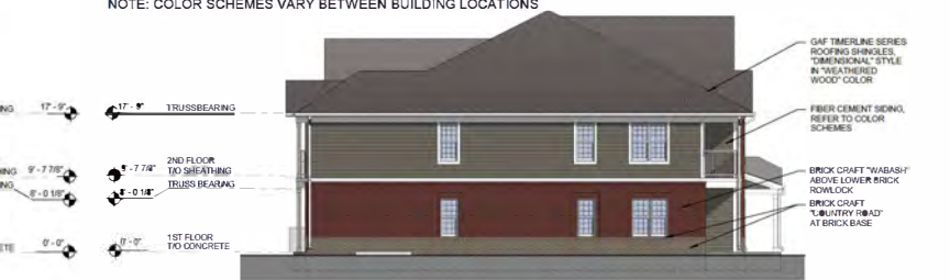
3 BUILDING TYPE 12B LEFT ELEVATION 1/8" = 1'-0" BUILDINGS 2, 6, 7, 10, 12, & 16
