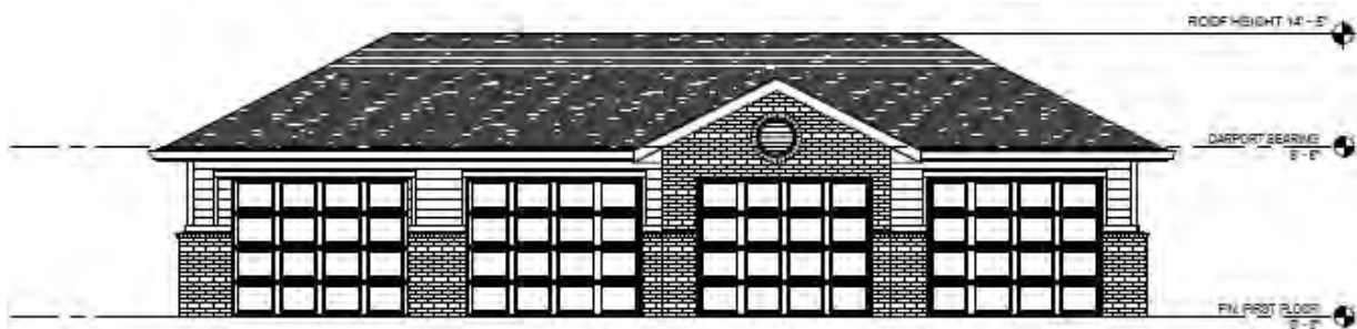
② GARAGE REAR ELEVATION - 4 BAY STANDARD 3/16" = 1'-0"
