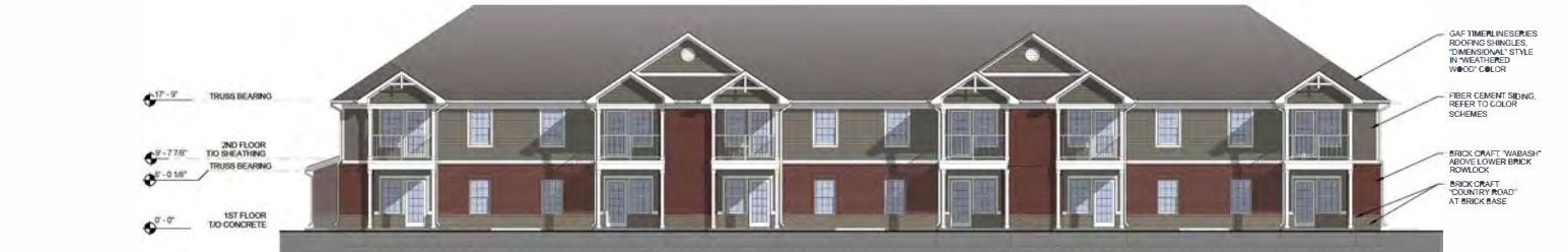
2 BUILDING TYPE 12B REAR ELEVATION 1/8" = 1'-0" BUILDINGS 2, 6, 7, 10, 12, & 16
