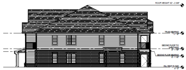
4 BUILDING TYPE 12C RIGHT ELEVATION 1/8" = 1'-0"
