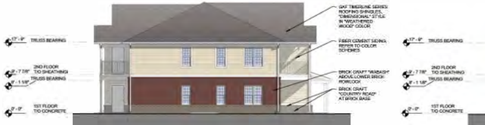
3 BUILDING TYPE 12A LEFT ELEVATION 1/8" = 1'-0" BUILDINGS 3 & 4
