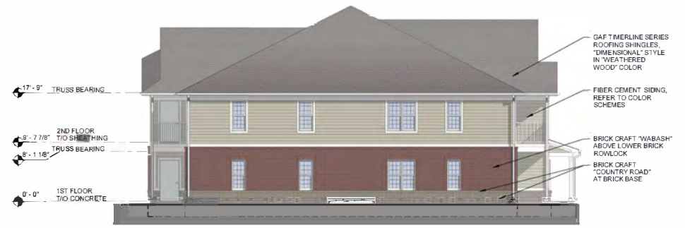
3 BUILDING TYPE 12C LEFT ELEVATION 1/8" = 1'-0" BUILDINGS 8, 9, & 11
