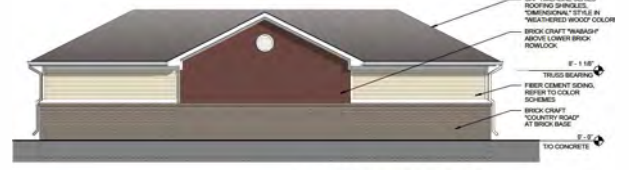
2 GARAGE REAR ELEVATION 3/16" = 1'-0"
