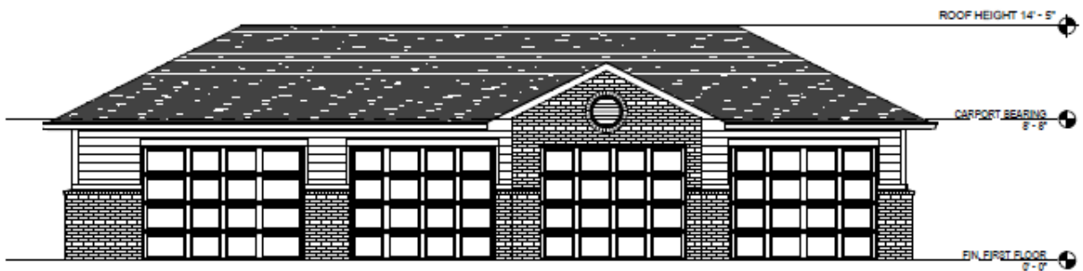
② GARAGE REAR ELEVATION - 4 BAY HC 3/16" = 1'-0"
