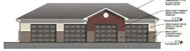
1 GARAGE FRONT ELEVATION 3/16" = 1'-0"
