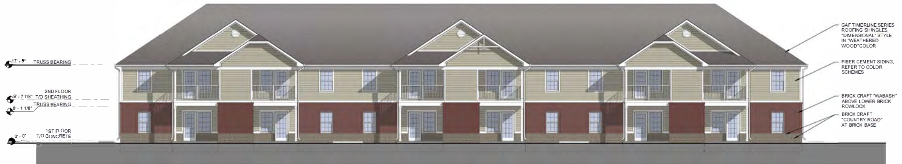
2 BUILDING TYPE 12C REAR ELEVATION 1/8" = 1'-0" BUILDINGS 8, 9, & 11
