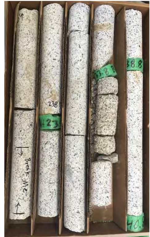
Granitic Bedrock Cores Boring B-09, 20.5 to 40.8 Feet
