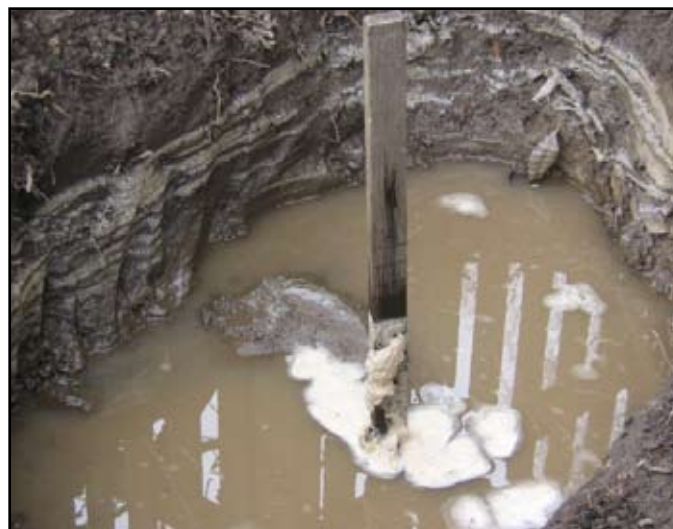
Use a ruler to measure the rate of infiltration in a pit.
