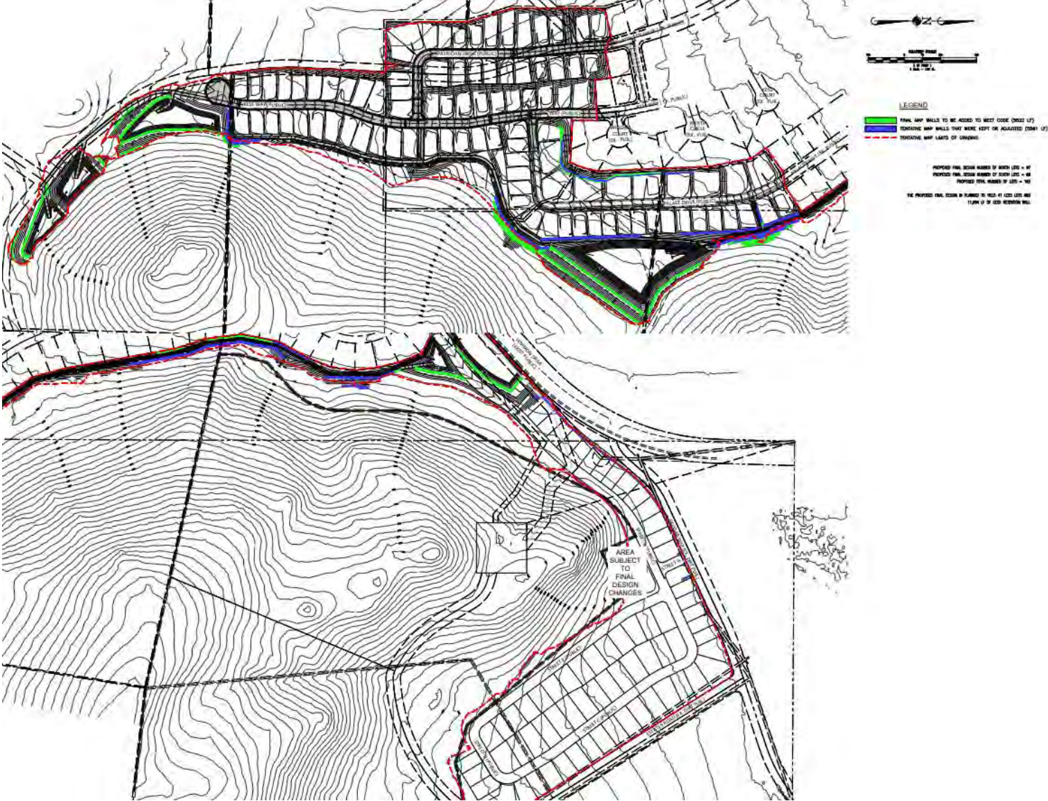
Figure 3: Proposed Final Map Retaining Walls Comparison (full size provided with application materials)
