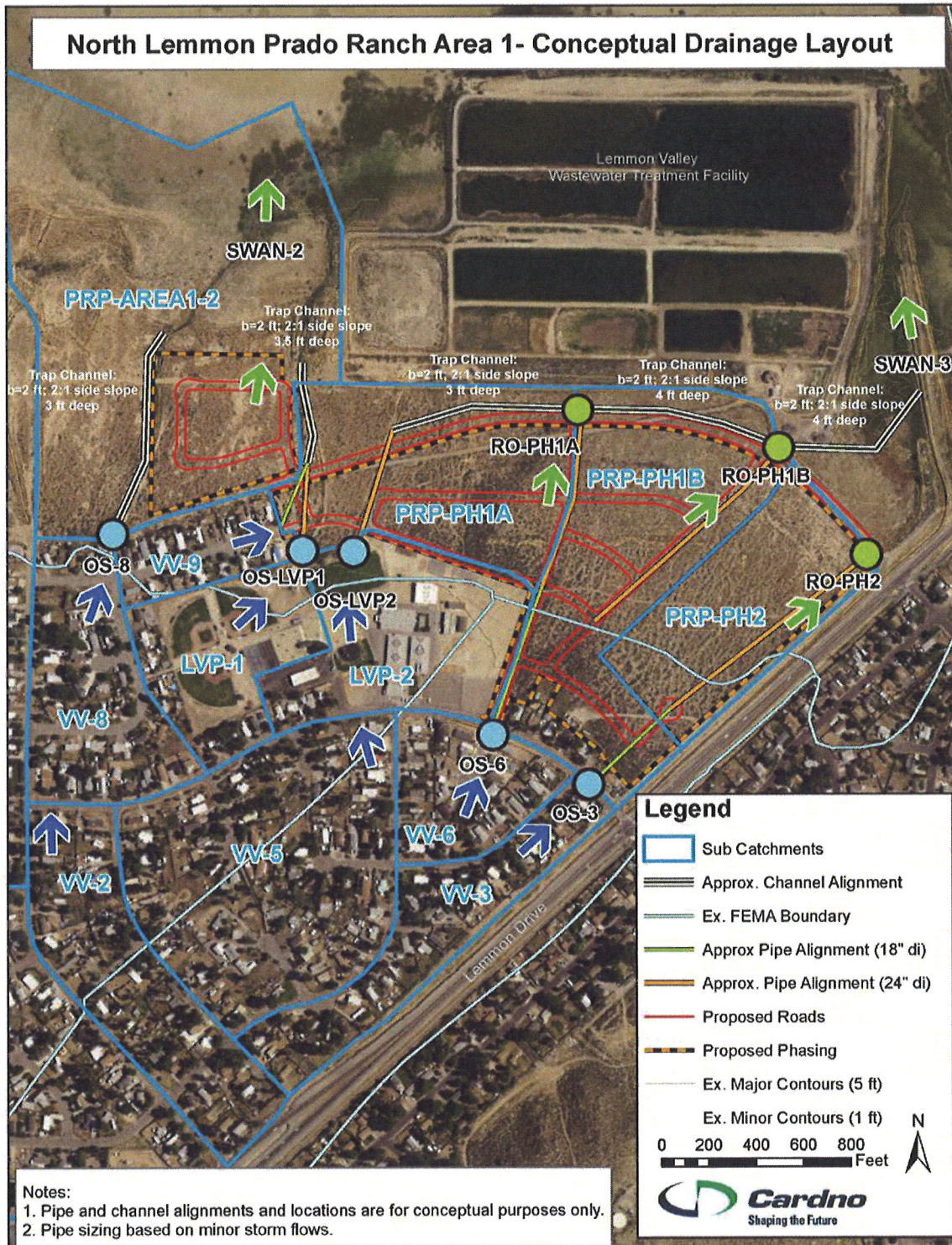
Figure 7. Conceptual drainage plan for the proposed Area 1 development.
