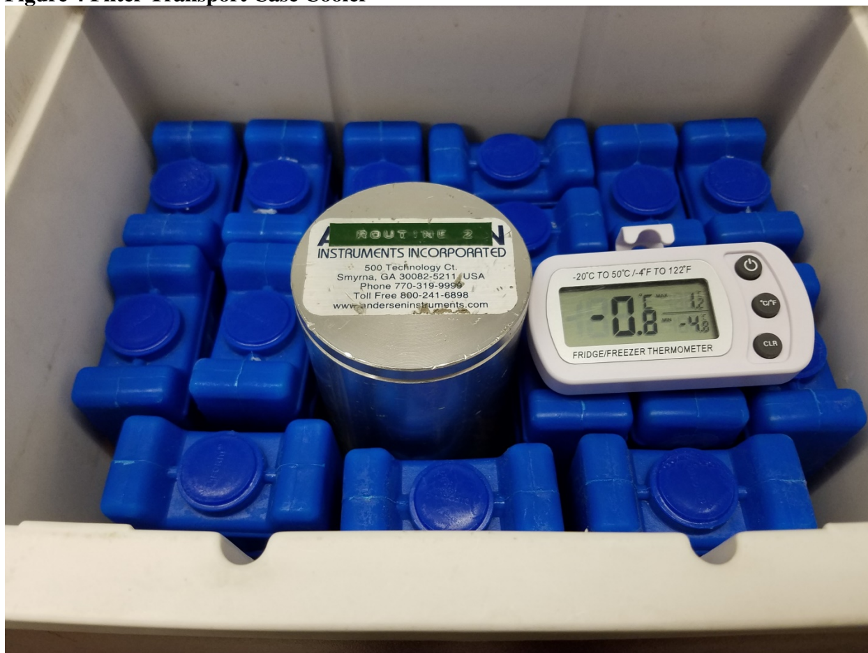
Figure 4 Filter Transport Case Cooler
