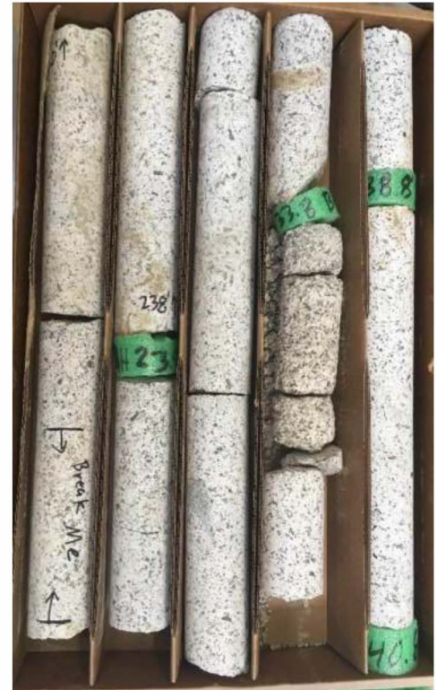
Granitic Bedrock Cores Boring B-09, 20.5 to 40.8 Feet
